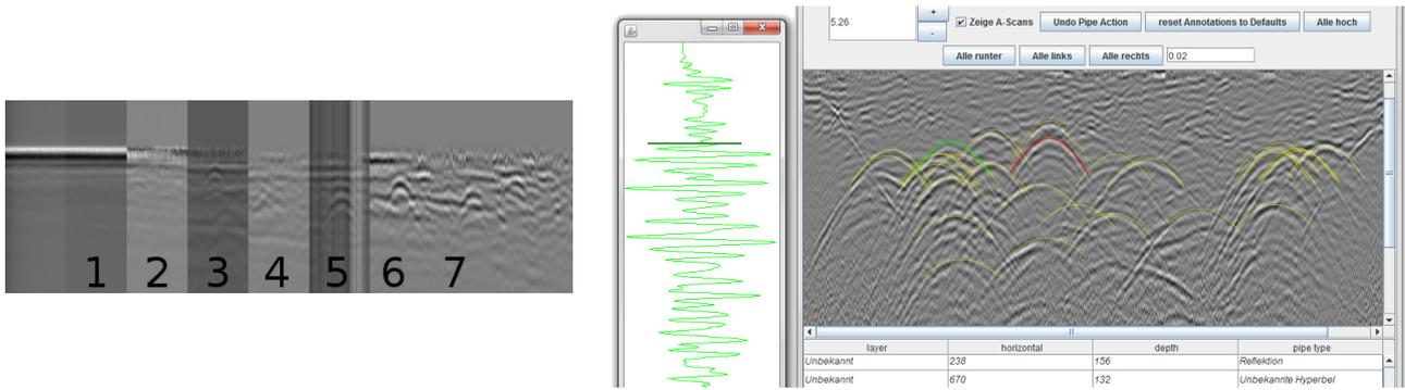
Figure 2: Our GPR Analyzer and Annotator preprocesses data as shown on the left. After preprocessing, a GUI shows basic information on individual pipes / hyperbolas and is used to interactively perform CRUD - Create, Retrieve, Update and Delete - operations for hyperbolas.
