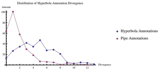
Figure 4: Inter human analysis of annotation behavior: The absolute differences exceed 12 hyperbolas (not shown here), resulting in diverging model performances at a later stage.
